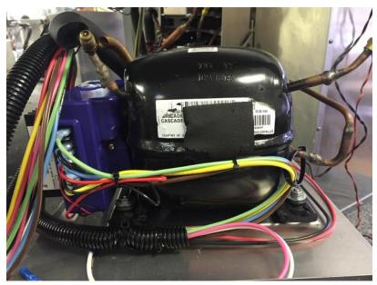
All Medi-Kool Climate Controlled Cabinets are compressor based. We use a Masterflux Cascade Compressor, as seen in the image above. This photo shows a compressor assembly with the matching electronic module. All of our units are operated with one size compressor. Each compressor is mounted to the unit at the customers specification (rear, right, left or top).
