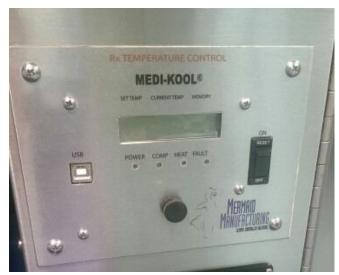
The Medi-Kool board maintains temperatures within one degree of your set perimeter. Our control boards require a 4 minute delay in order to regulate the compressor. These boards can maintain temperatures as low as 32 degrees F or as a high as 110 degrees F. Beginning 2015, new manufactured boards have the ability to read Celsius as well as come in our stainless finish (as shown in this photo).
