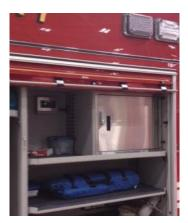
This unit is designed to hold extremely large drug bags. In the picture above, you can see the unit mounted on the side of a fire truck. Compressor can be mounted rear, right, left or top. Adjustable vented shelf is included. Door can be hinged right or left.
