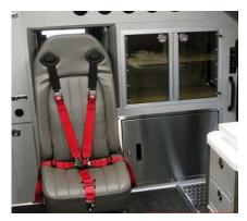
Similar to the MK 747 SS, this cabinet has the same height. The difference is that this unit is 3" wider and 10" deeper. Compressor can be mounted rear, right, left or top. Adjustable vented shelf included. Door can be hinged right or left.
