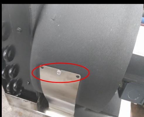
**Step 6** is to reattach the rear brackets. <u>Make sure the blower is firmly against</u> the shroud with no gap between them, or it will suck in warm air, bypassing the <u>evaporator</u>.
