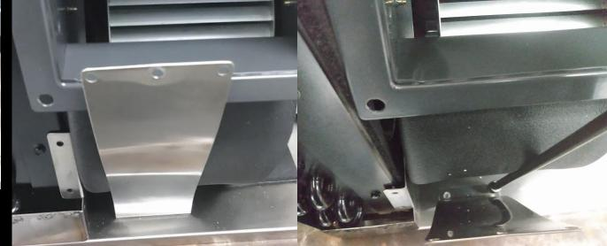
**Step 7** is to reattach the condenser. Once the screws are in, reach in and spin the blower wheel, to make sure none of the screws have jammed it. If jammed or scraping, you can loosen the screws until the touching screw is found. The touching screw can be backed out a few threads until it is no longer touching, or removed completely as long as the condenser is still firmly in place.
